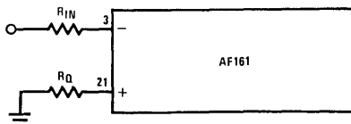
FIGURE 6. Connection for Any Q, Inverting
